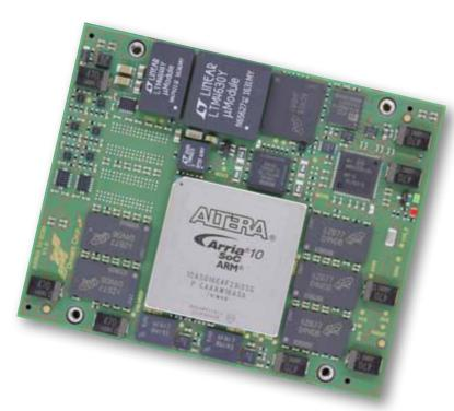
The Arria 10 SoM was developed with an emphasis on embedded and automotive vision applications. Using Intels Arria 10 SoC devices in the 29x29 mm package, the module off ers a multitude of interfaces in a small 8 cm by 6.5 cm form factor.
